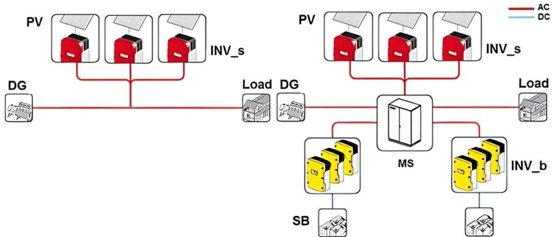
**Fig. 1.** Operating schemes of isolated energy systems: (a) parallel operation of diesel power plant and photovoltaic system; (b) isolated energy system with battery energy storage system, diesel generator works as an emergency energy source ([www.sma.de](http://www.sma.de)).
