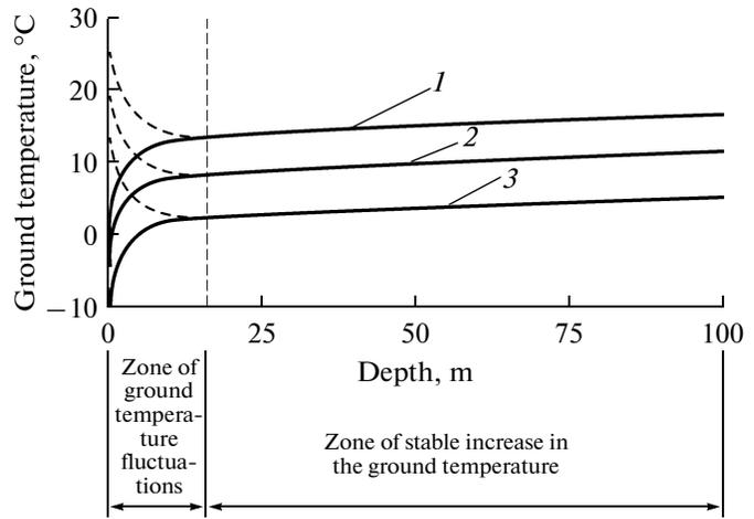
Fig. 6. Distribution of the ground temperature in depth (with an account for seasonal fluctuations). (1) South; (2) Center; (3) North; — winter; --- summer.
