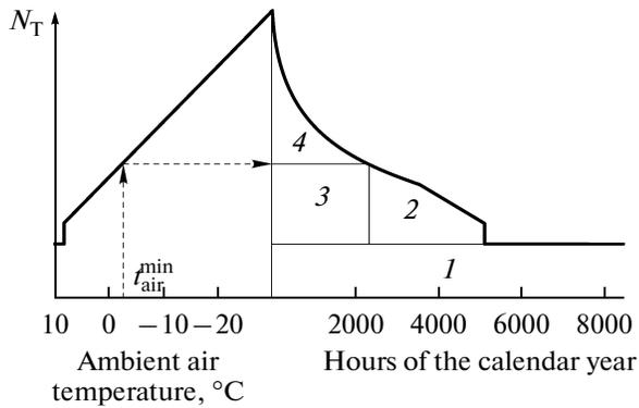
Fig. 4. Zones of HPU operation at the diagram of heat loads duration.
