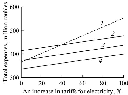
**Fig. 7.** Effect of an increase in tariffs for electricity and a decrease in specific capital investments for HPUs ( $\Delta K$ ) on competitiveness of HPU relative to electric boilers while supplying heat to cottage settlement (Central region). (1) electric boiler; (2)–(4) HPU;  $\Delta K$ , %: (2) 0; (3) 20; (4) 40.
