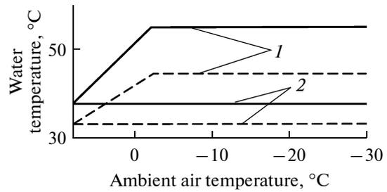
**Fig. 3.** Temperatures of direct and return water in parallel schemes of heating with HPU (for the conditions of Moscow). (1) system with radiators; (2) "warm floor" system; — direct water; --- return water.
