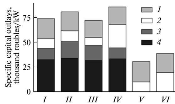
Fig. 5. Specific outlays in alternative versions of heat-supply (for the conditions of Moscow). (I) HPU with redundant electric boiler (EB) (90/70°C temperature schedule); (II) HPU with redundant EB (70/50°C schedule); (III) HPU with peak convector; (IV) HPU with “warm floor” system and peak EB; (V) one EB; (VI) one gas boiler; (1) substation, gas-distribution station; (2) electric or gas boiler and radiators; (3) drilling; (4) HPU with assembling works.
