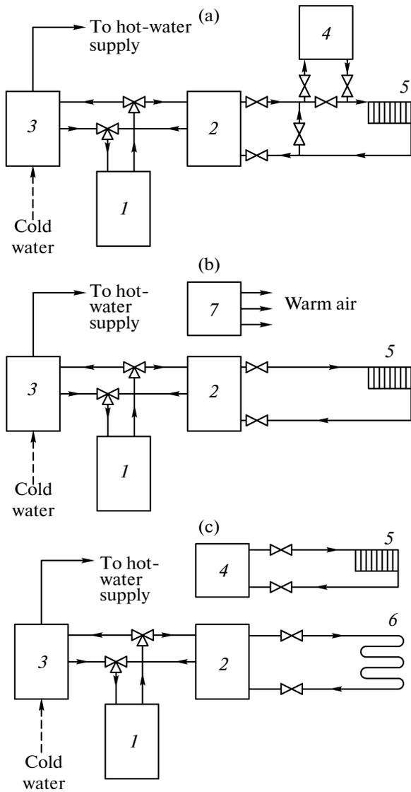
**Fig. 2.** Heat-supply schemes for individual house with HPU. (a) Series scheme with electric boiler; (b) parallel scheme with radiators and convector; and (c) parallel scheme with "warm floor" and electric boiler. (1) heat pump; (2) intermediate tank; (3) accumulating water heater for hot-water supply; (4) electric boiler; (5) heating system with radiators; (6) "warm floor" heating system; (7) electric convectors.
