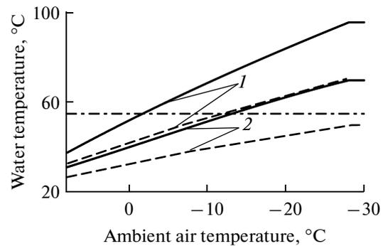
**Fig. 1.** Dependence of direct and return water temperatures in the heat supply systems on the ambient air temperature (the conditions of Moscow). (1) High-temperature system (95/70°C); (2) low-temperature system (70/50°C); — direct water; --- return water; ···· maximum water temperature at the outlet from HPU.
